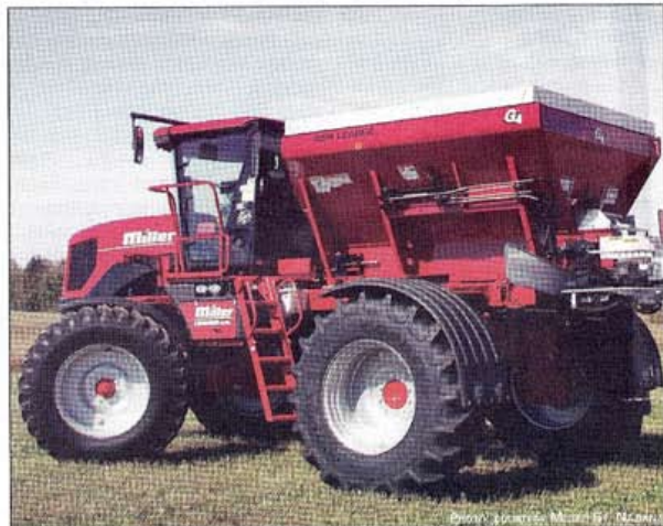
New for Miller St. Nazianz's Condor line of mechanical-drive sprayers is a 255 cubic-foot capacity dry spreader box.
